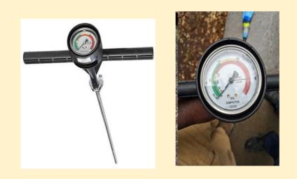
Soil compaction using a Dickey-John Tester
